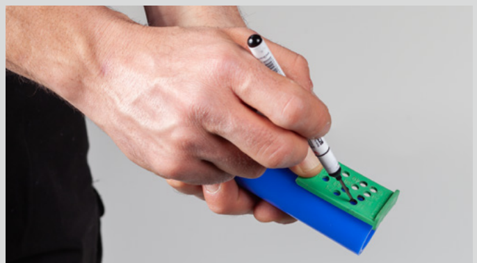
Marking of the welding depth
