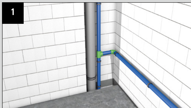
Positioning of the fixed point clamp
