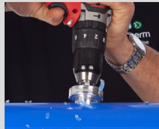
Removal of the oxygen barrier layer in case of the aquatherm blue pipe OT and of the UV layer in case of the aquatherm UV-pipe
