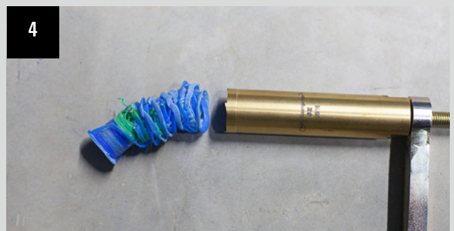
4. Removal of the drilling residues out of the drilling tool
