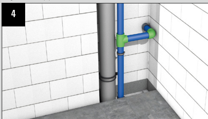
Installation of a spring leg
