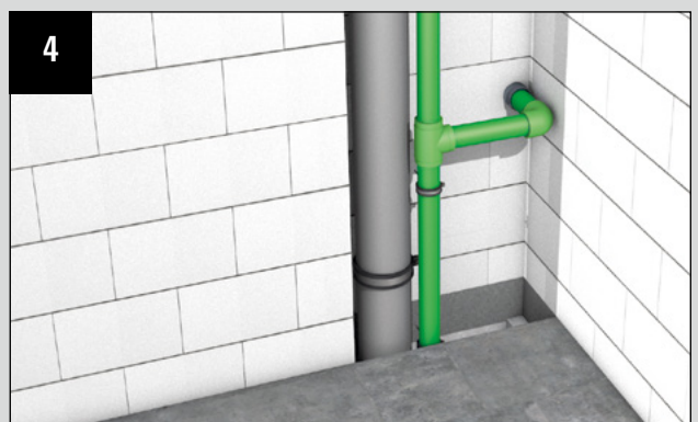
Installation of a spring leg
