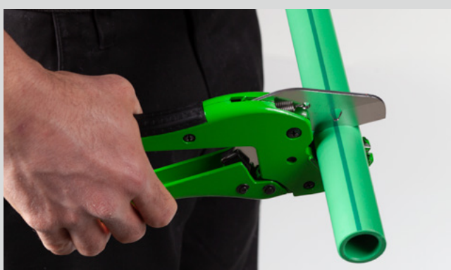
Cutting of the pipe
