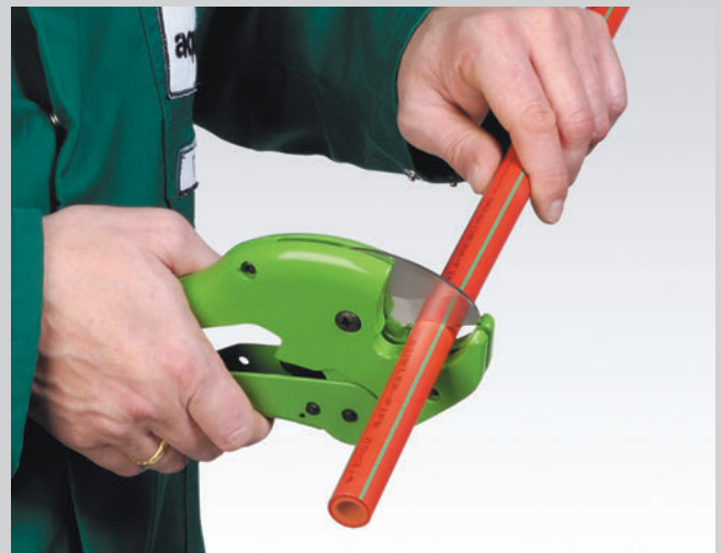
Cutting of the pipe
