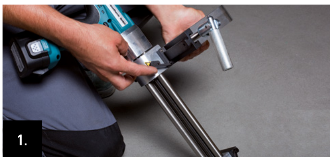
1. Adjust pipe slide in the back guide rail to the required pipe dimension and fix with locking bow.
