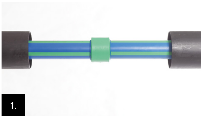
1. Preparation: Dry and clean the entire sealing area with a grease and lint-free cloth.
