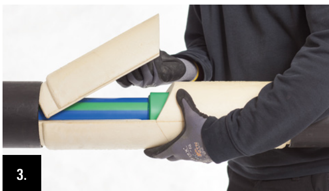
3. Insert the other PUR-insulation shells marked 1 and 2 as described. The tongue and groove profile of the shells ensures a gap-free and accurate joining.
