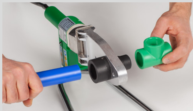
Heating-up of pipe and fitting
