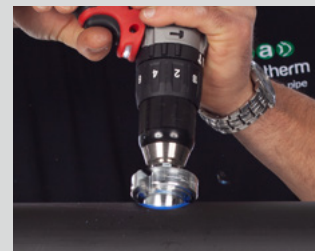
Removal of the oxygen barrier layer in case of the aquatherm blue pipe OT and of the UV layer in case of the aquatherm UV-pipe
