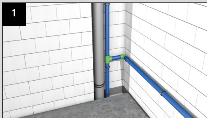
Positioning of the fixed point clamp
