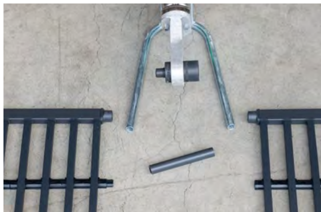
1. Welding device and tool (16 mm) mounted; temperature control performed.
