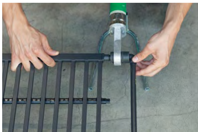
2. Insert elbow 90° female/male (16 mm) into the tool bushing and at the same time push the heating grid socket onto the heating spigot.
