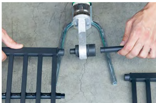
3. After the prescribed heat-up time of 5 seconds, pull the parts off the tools ...
